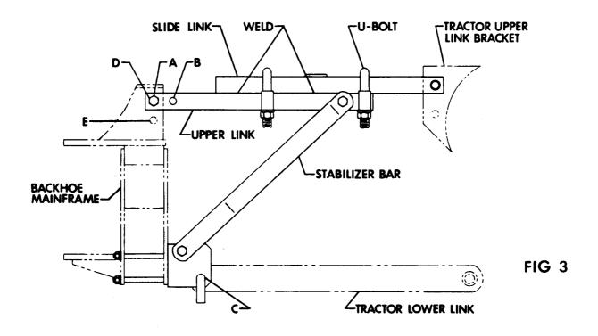
1. Attach lower link mounts (22, 23) to backhoe mainframe using eight bolts, locknuts, and flat washers (1, 4, 9) as shown in Fig 3 and 4. Torque to 50 ft-lb.
